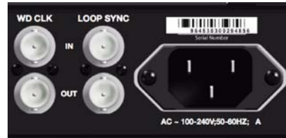
Back panel Word Clock and Loop Sync In and Out
