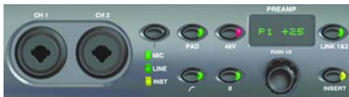
CH 1 and CH 2 MIC/LINE/DI Inputs, and Preamp controls
