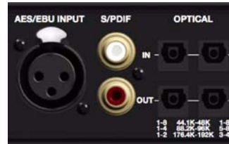
Back panel digital inputs and outputs
