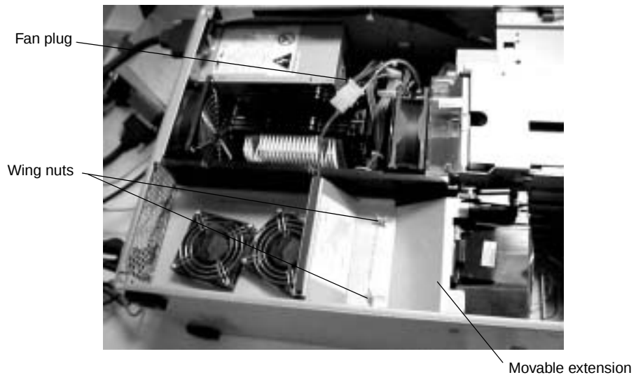
Figure 4-11 Fan in the System
