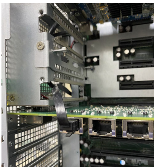
Example cable routing and connection to an MLN-192 card in EXPANSION slot 1 of an E6L-112 (shown at left) and important clearance for the side panel (shown at right)
