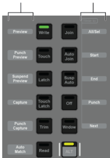
Advanced Automation switches on the Dock
