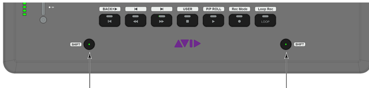
Dock Surface SHIFT switches
