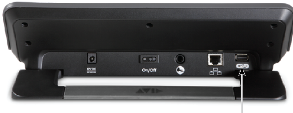
USB charging port on the back of S1
