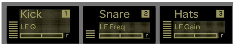
Channel displays in Channel Mode, showing “Kick” as the attentioned track
