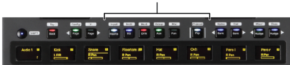
Channel Encoder Assign switches (showing all switches lit to indicate primary LED colors)
