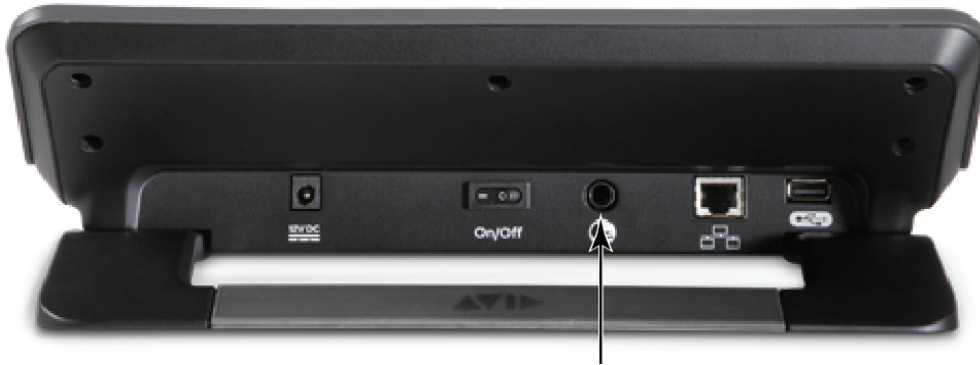
Footswitch input on the back of S1
