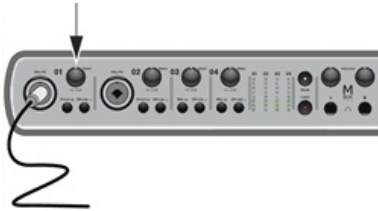
Input 1 Gain on Mbox Pro
