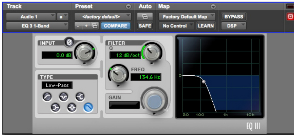
1-Band EQ set to Low Pass Filter
