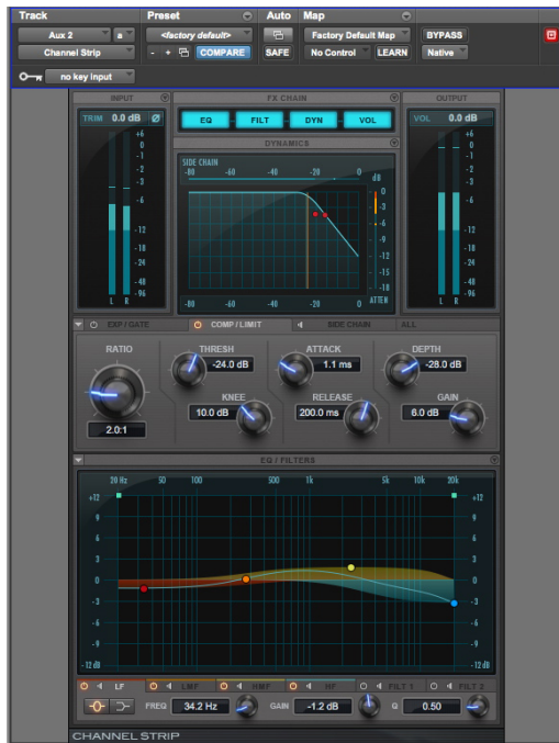
Channel Strip, Compressor / Limiter tab shown
