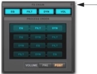
Showing the FX Chain Process Order
