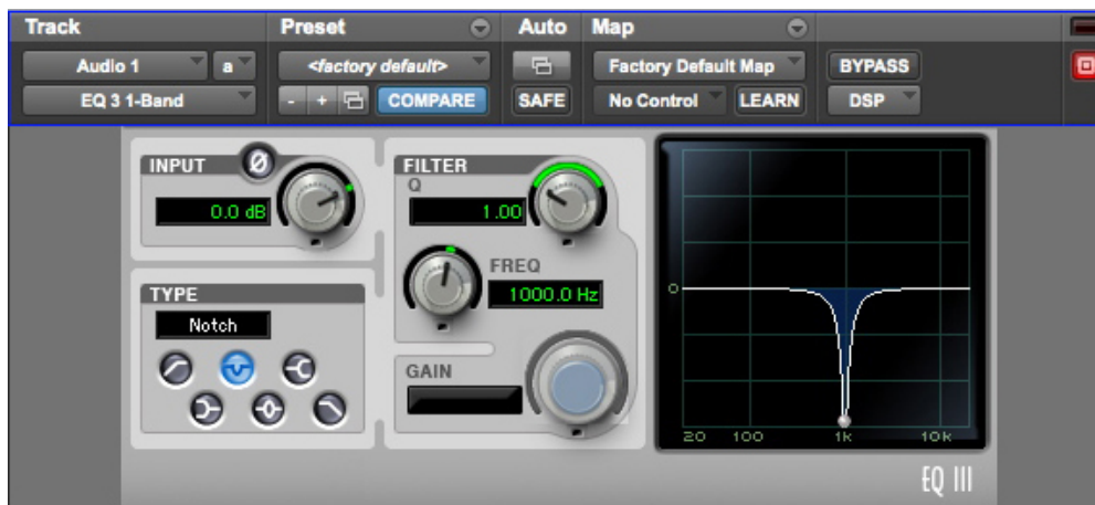
1-Band EQ set to Notch Filter
