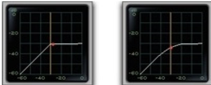
Graph examples of hard knee (left) and soft knee (right) compression
