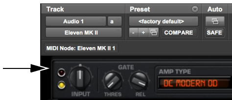
Eleven MK II's Input LED (top) and Clip LED (bottom)
