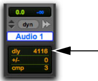
Determining the DSP delay of track inserts (Mix window shown)
