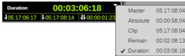
The following illustration shows the display for a sequence loaded in Output mode. Note that the smaller display also shows the duration of the sequence.
