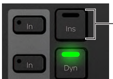
Inserts switch on Process Module
