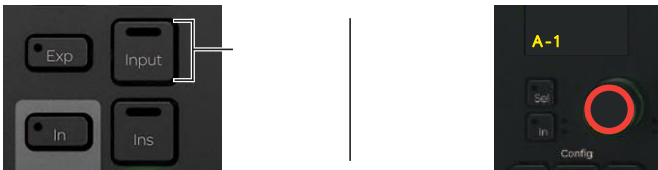
Figure 3. Input switch on Process Module (at left) and top level input knob set (at right)
