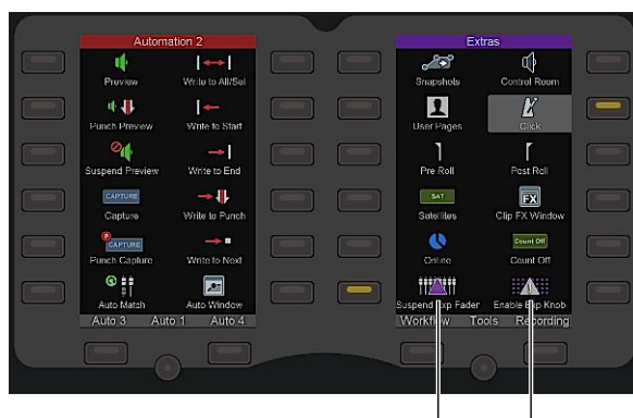
Figure 50. Automation Module Soft Keys showing Attention Expand Faders enabled and Attention Expand Knobs disabled
