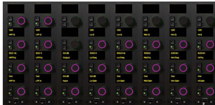
Figure 48. Attention Expand Knob Zone with expanded EQ3 7-band (plug-in bypass via column 8 Back switch)
