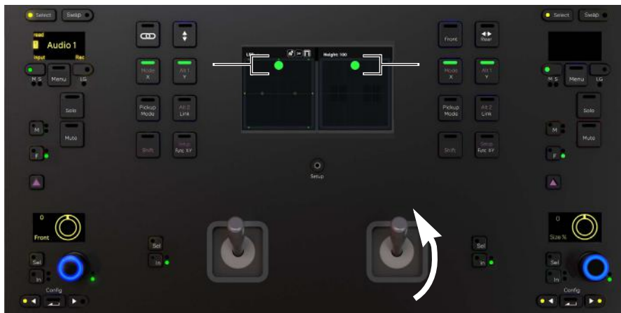
MJM panner grid in Height Adjust mode; the same mono track at front/center, but Height at maximum (100) / joystick 2 all the way up
