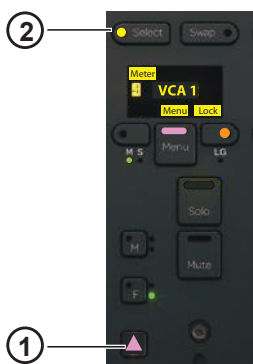
Attention (1) and Select (2) on a Fader Module
