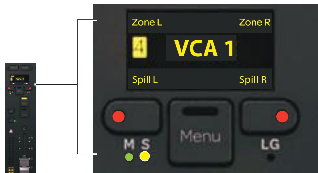
Figure 21. Spill controls and indicators when Menu switch is pressed, showing a VCA slave (S indicator LED lit yellow)
